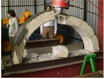
Figure 4. Collapse of the second reinforced arch.
